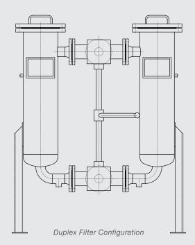
For continuous operation, Duplex Filter consisting of 2 single bag filters are connected together with a 3-way influent and effluent valve. Each single bag filter can be operated on alternate basis and bag change done during the filter on stand-by for continuous production flow.
